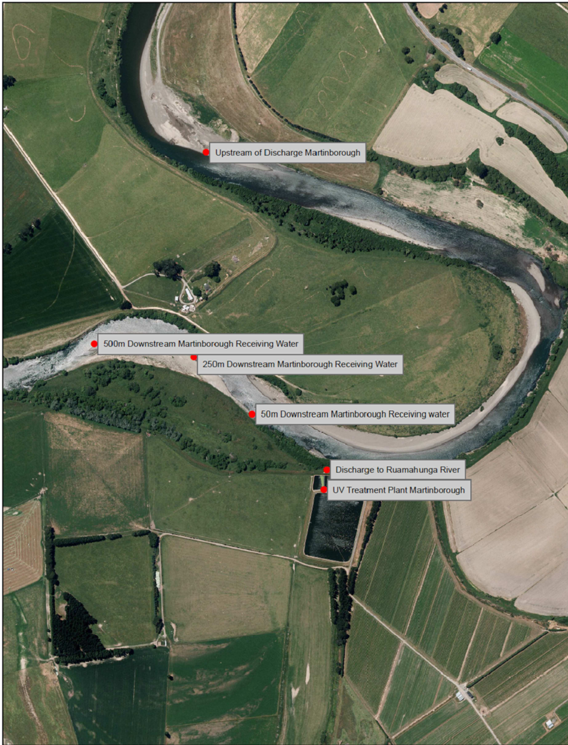
Figure 1: Indicative monitoring site locations (NB Inlet monitoring location to be confirmed upon installation of equipment during Stage 1A).
