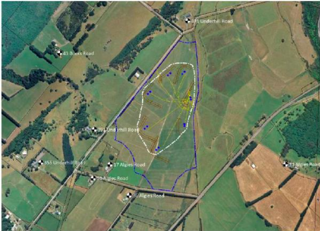
Figure 3: Map showing where bunding is required, and where no crushing or screening works can occur to meet noise limits.
