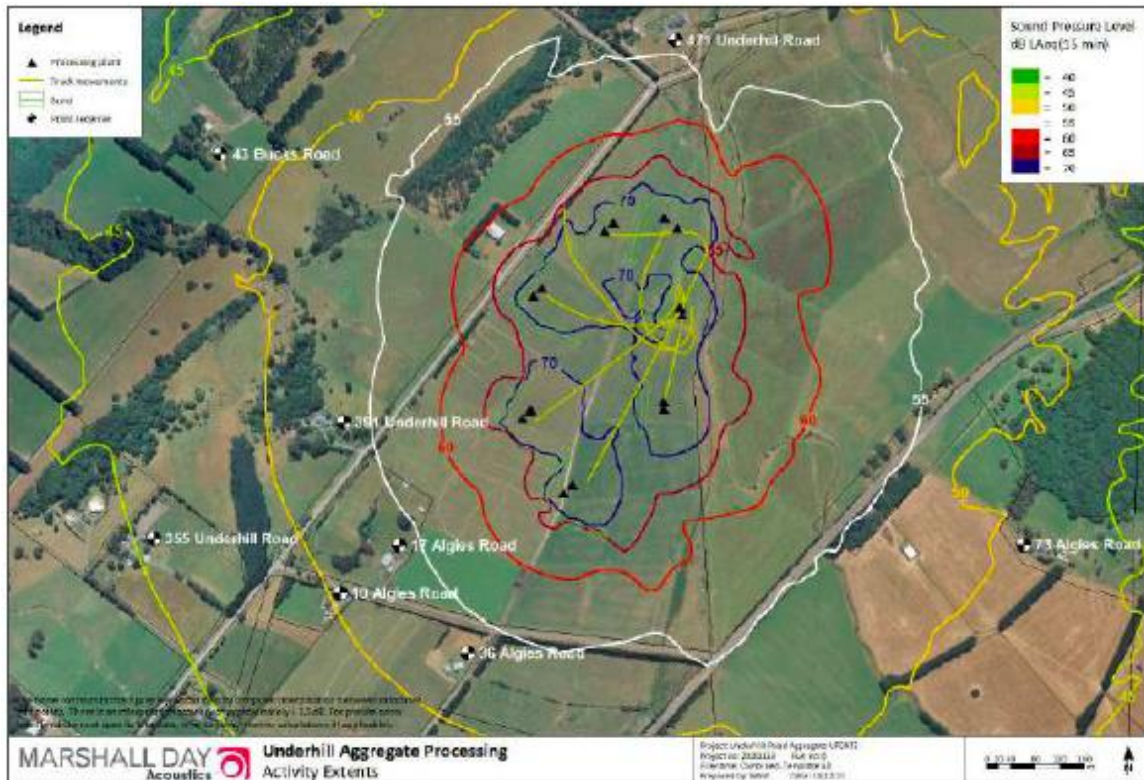
Figure 5: Noise contours from all potential crusher sites (aggregated), undertaken by Marshall Day in response to questions posed by the peer review
