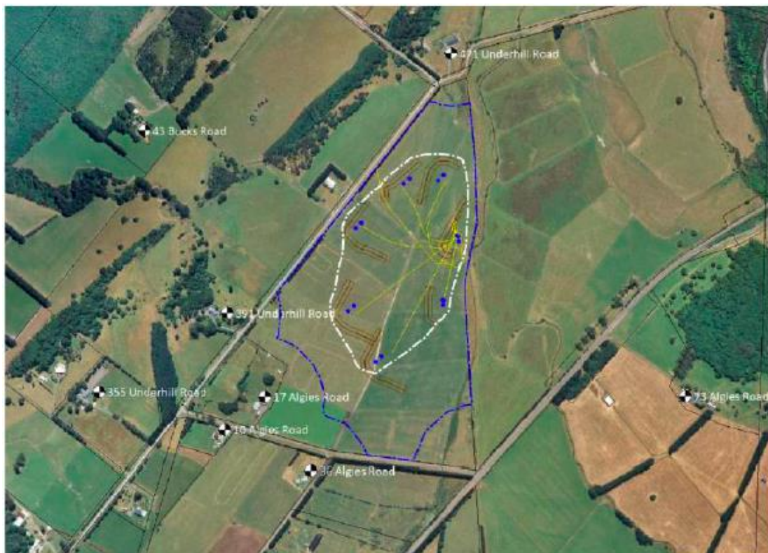
Figure 1: Site plan showing extent of extraction areas (blue line), processing areas with bunds (white dotted line), and central crusher site within the bunds on the subject site
