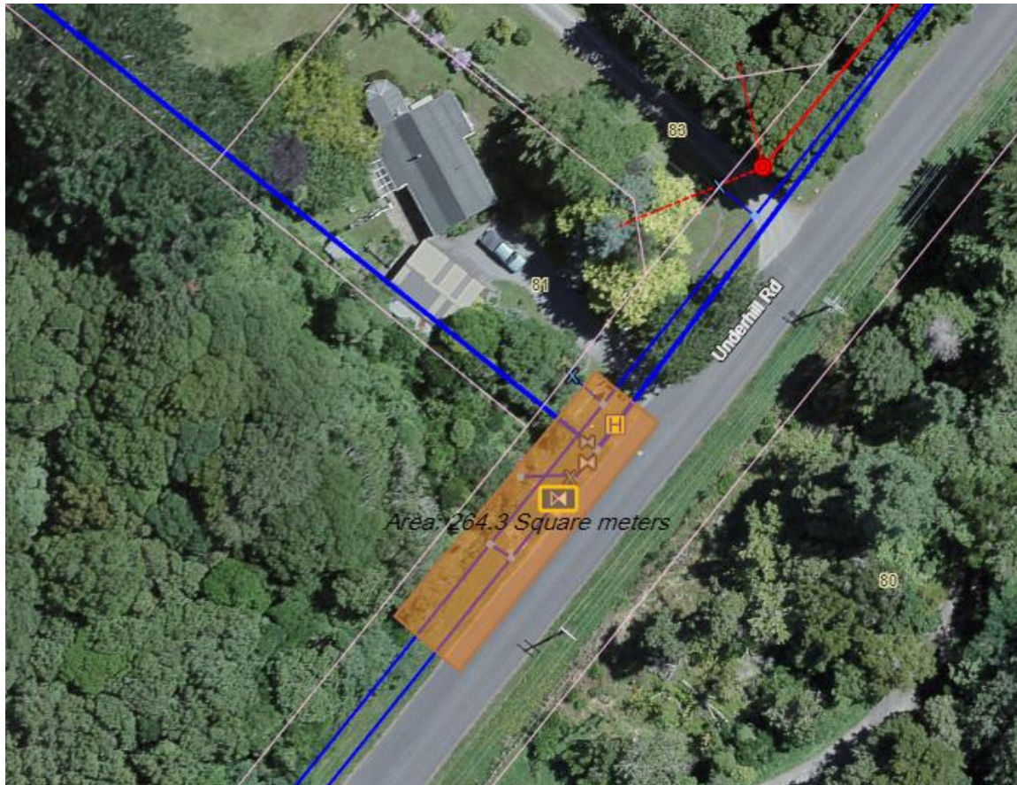
Figure 9: Proposed location for network reticulation distribution arrangement via pumping to reservoir, and approximate extent of pump setup in orange. (Asset data and aerial from Wellington Water Regional Water Stormwater Wastewater App (23/11/2021))
