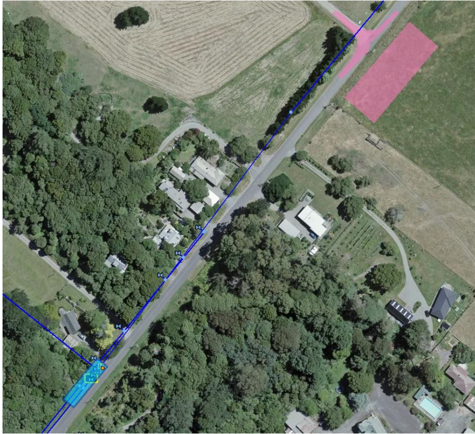
Figure 7: Possible water pump setup location at 81 Underhill Road in blue and subsequent proposed turning bay area in the reserve (1320m 2 , 22m x 60m). Approximate hydrant location in orange. (Asset data from Wellington Water Open Data Portal (23/11/2021). Aerial from LINZ – South-wairarapa urban 2021 0.075m & others 2020-2021)
