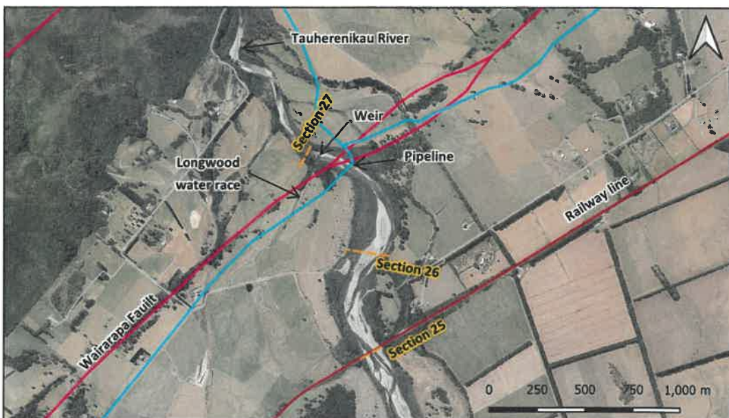
Figure 1: Location of the pipeline crossing
