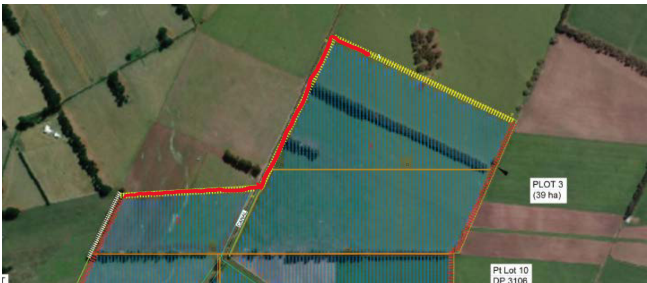
Figure 1 - proposed location of 2m height planting at implementation to mitigate potential effects of glare on State Highway
