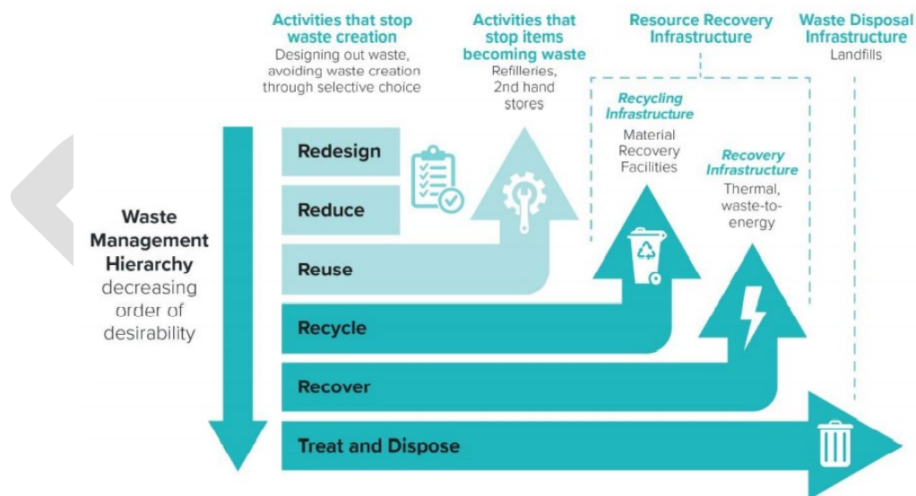
Figure 12 Waste minimisation hierarchy and resource recovery and disposal infrastructure (Te Waihangā, New Zealand Infrastructure Commission 2020, adapted from s44 Waste Minimisation Act 2008 and Auckland Council 2018) 24
