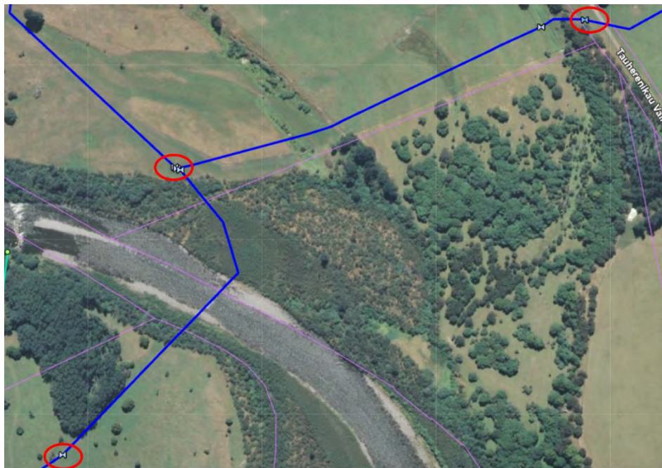
Figure 2: Isolation valves for river crossing pipeline (Wellington Water GIS 23/11/2021) Refer to Appendix 2 for location with respect to the Featherston town.
