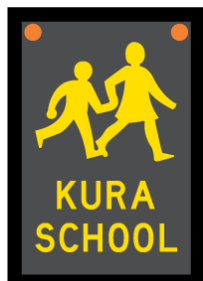
Figure 2.3: W19-2.1 Warning – symbol illuminated when activated (Kura School) — Permanent warning 3
