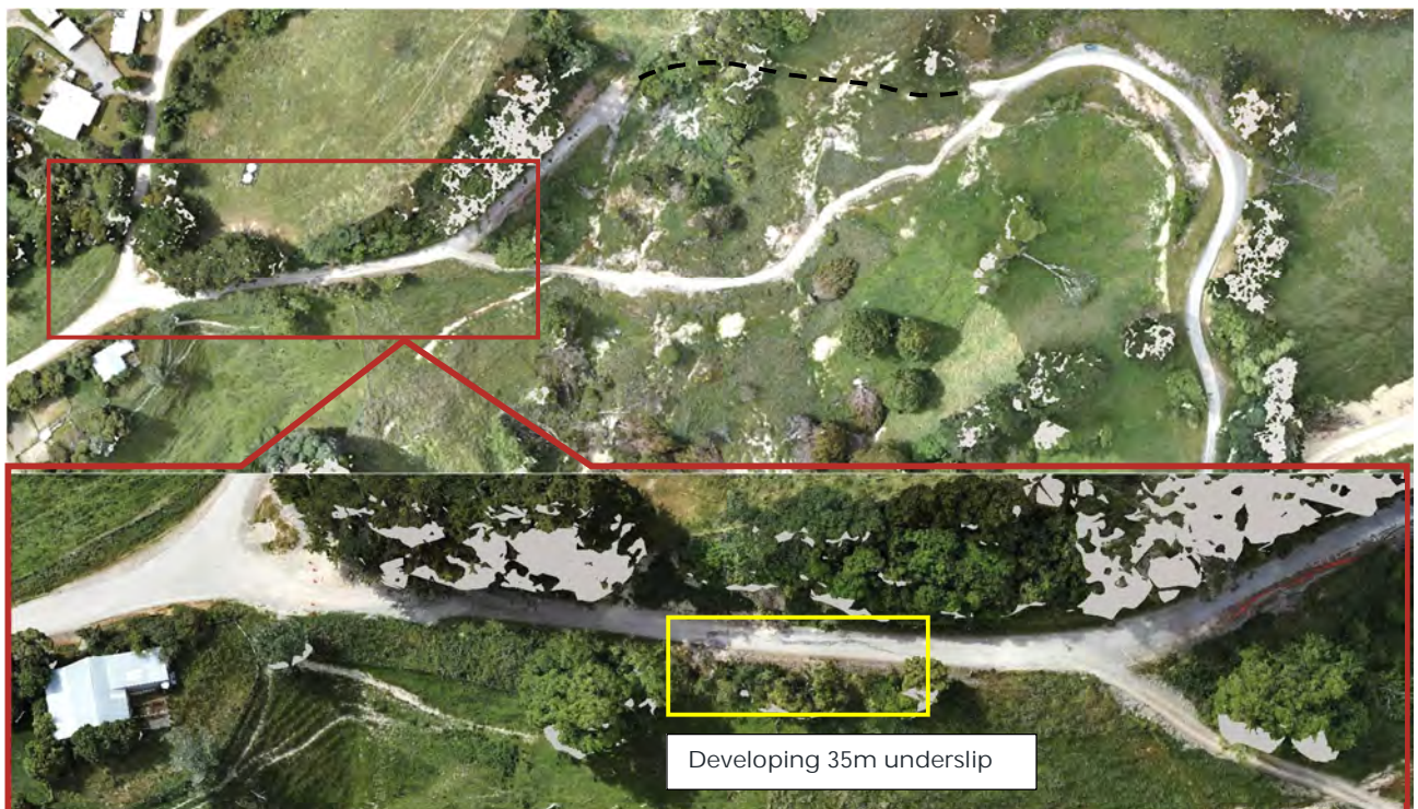
Figure 3: Underslip forming along Hinekura Road near Hikawera Road .
