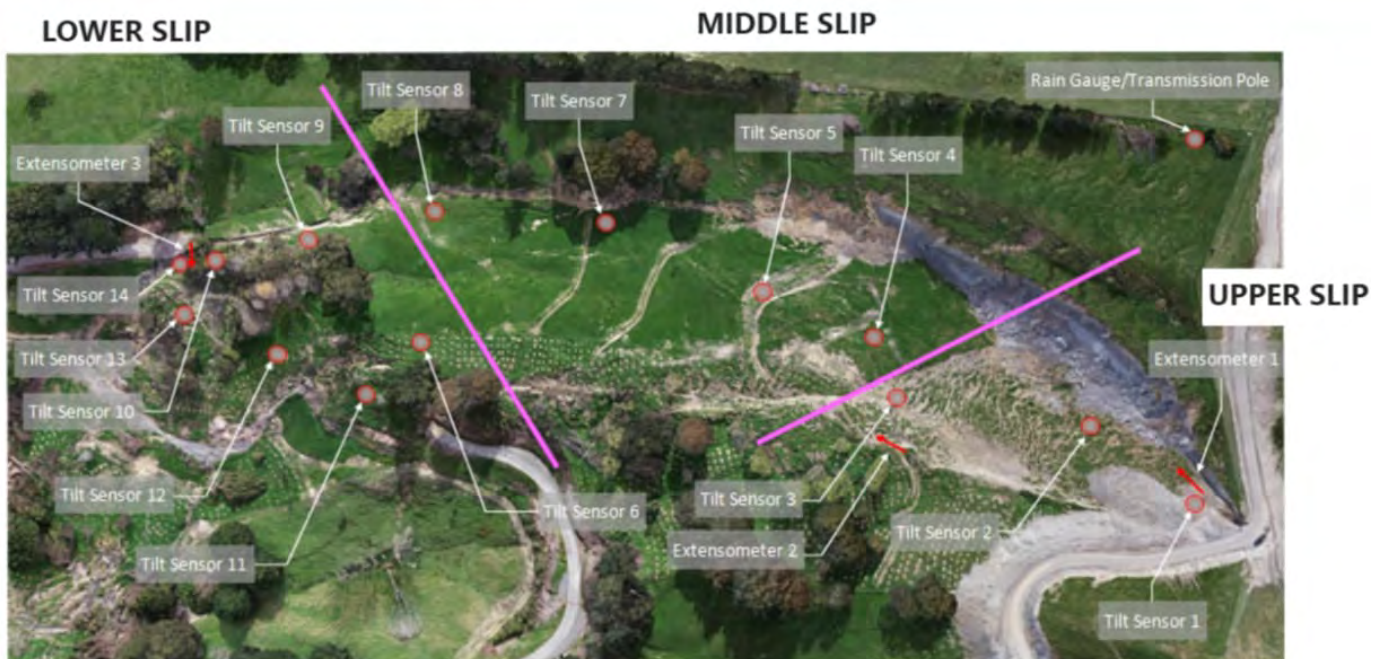
Figure 19: Remote monitoring network at Hinekura Road Landslide
