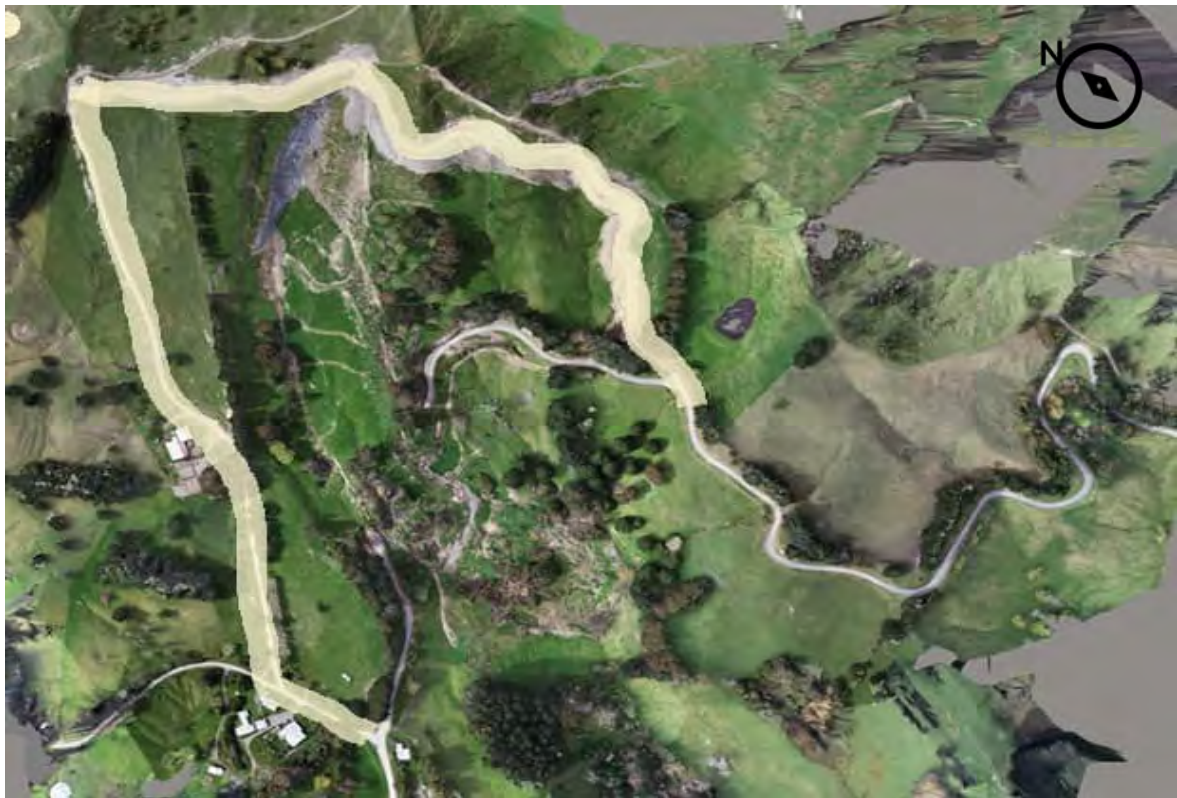
Figure 5: Temporary road constructed by landowners to bypass Hinekura Road landslide .
