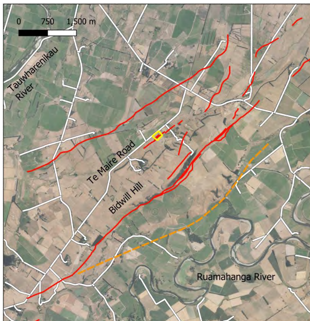
Figure 1 Overview map showing southern portion of Te Maire Fault. Red lines from GNS mapping by Litchfield et al. (2022), orange dashed line = inactive thrust fault from Nicol et al. (2002), site marked in yellow.
