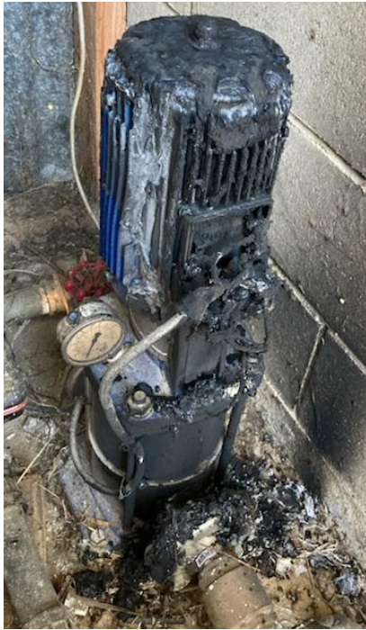
Figure 1. Burnt-out water pump, Martinborough
