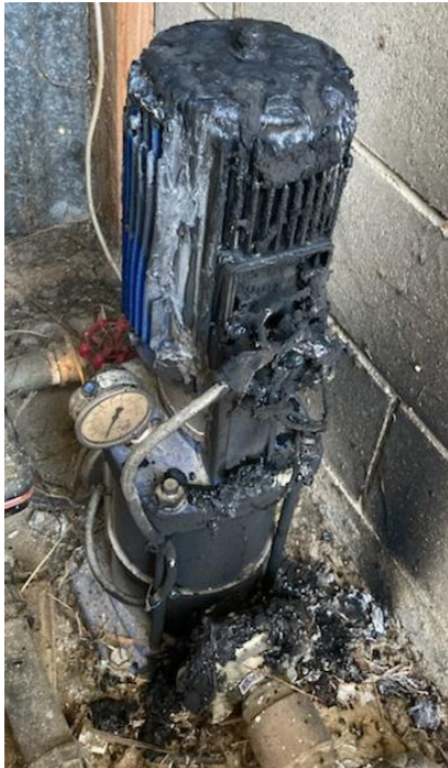
Figure 1. Burnt-out water pump, Martinborough
