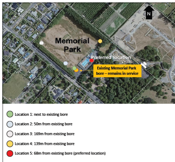
Figure 1: Bore Locations considered
