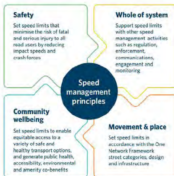
Figure 4.4: Guiding principles for speed management (Source: Waka Kotahi 10 )
