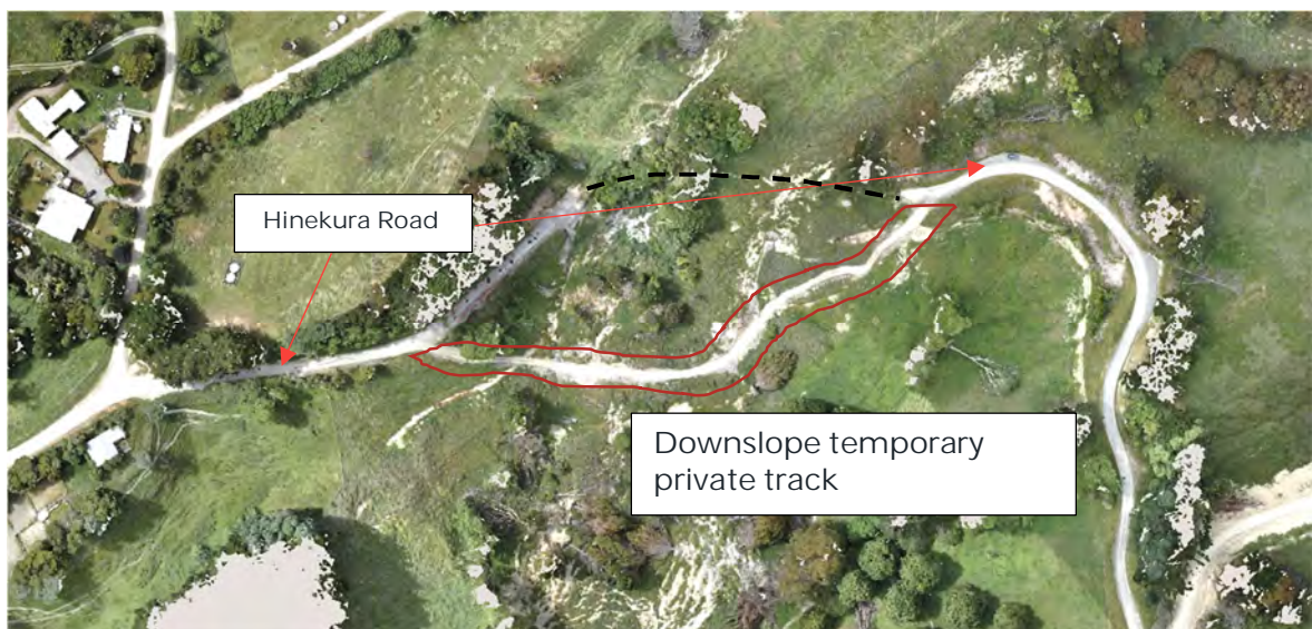
Figure 6: State of Hinekura Road in December 2022 with new downslope temporary track following remnants of old severely displaced carriageway.
