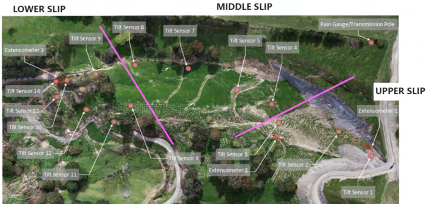
Figure 19: Remote monitoring network at Hinekura Road Landslide
