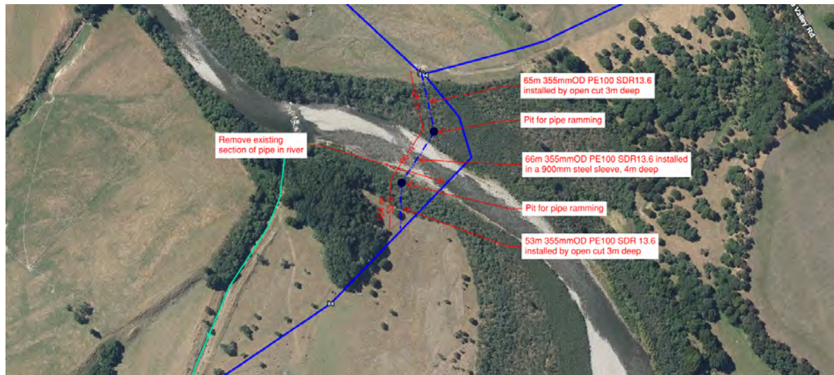
Figure 11 Option 3 – Trenchless Installation
