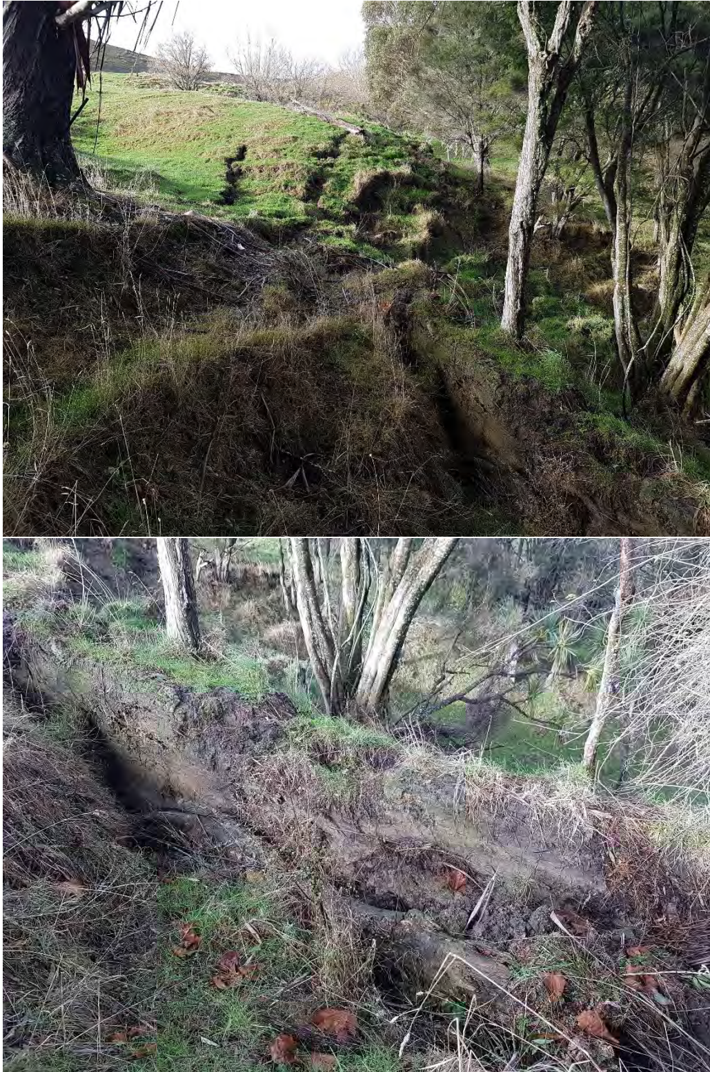
Eastern margin of landslide pushing steeper slopes below and causing secondary movement onto steeper slopes above road. Subhorizontal striae visible on both photos showing main movement is very low angle (near horizontal).
