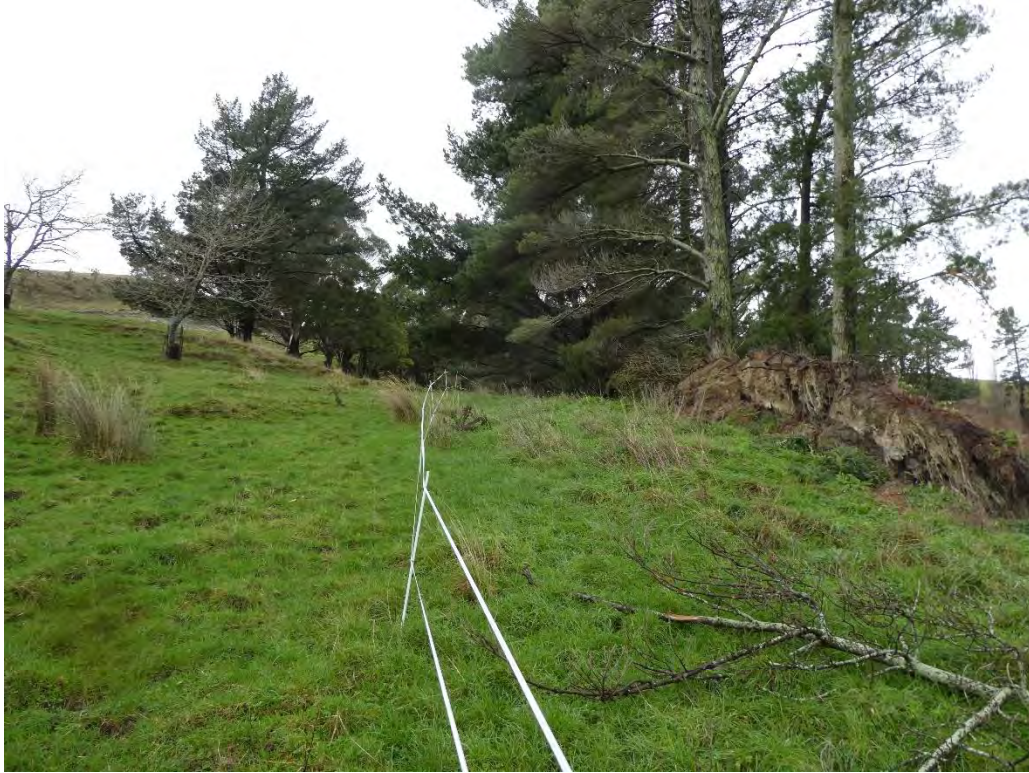
Lower slope above road landslide has pushed and tilted pine trees at top of steep slope above road (which have been cut down this week to the right – photo below)
