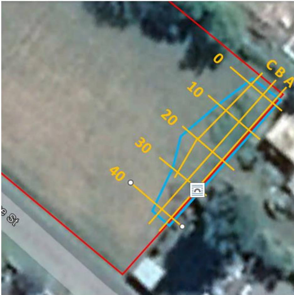
Figure 1 Remediated area and validation sampling grid
