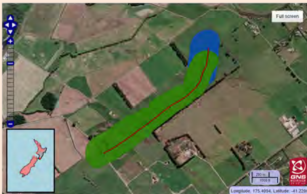
Figure 6: Fault lines (active trace in red, fault avoidance zones in green and blue)
