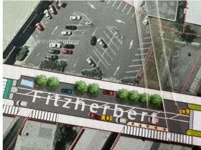
J) The trees shown as planted on either side of Fitzherbert Street will obscure sight lines for vehicles wishing to turn left when pulling out of LYONS Street (incorrectly noted as Birdwood Street on the plan). Vehicles needing to turn right from Lyons St will need to pull out further to be able to see west along Fitzherbert St, potentially exposing themselves to large vehicles travelling north at the same narrowed intersection, or those travelling south through same..
