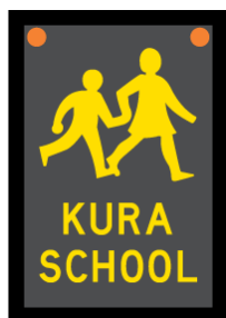
Figure 2.3: W19-2.1 Warning – symbol illuminated when activated (Kura School) — Permanent warning 4
