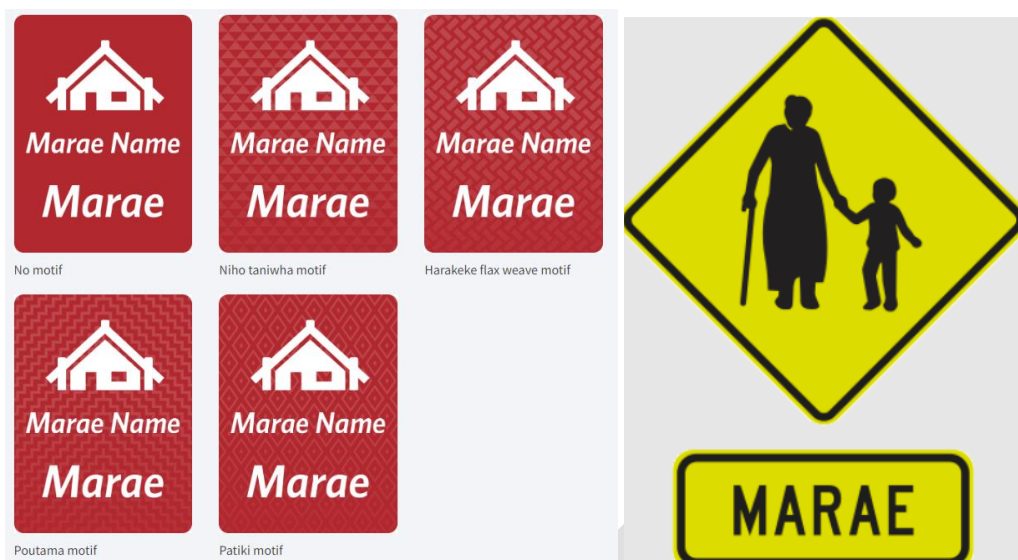
Figure 2.11: Options of cultural marae sign (left) and W16-11 marae warning and supplementary – pedestrians (right) 5
