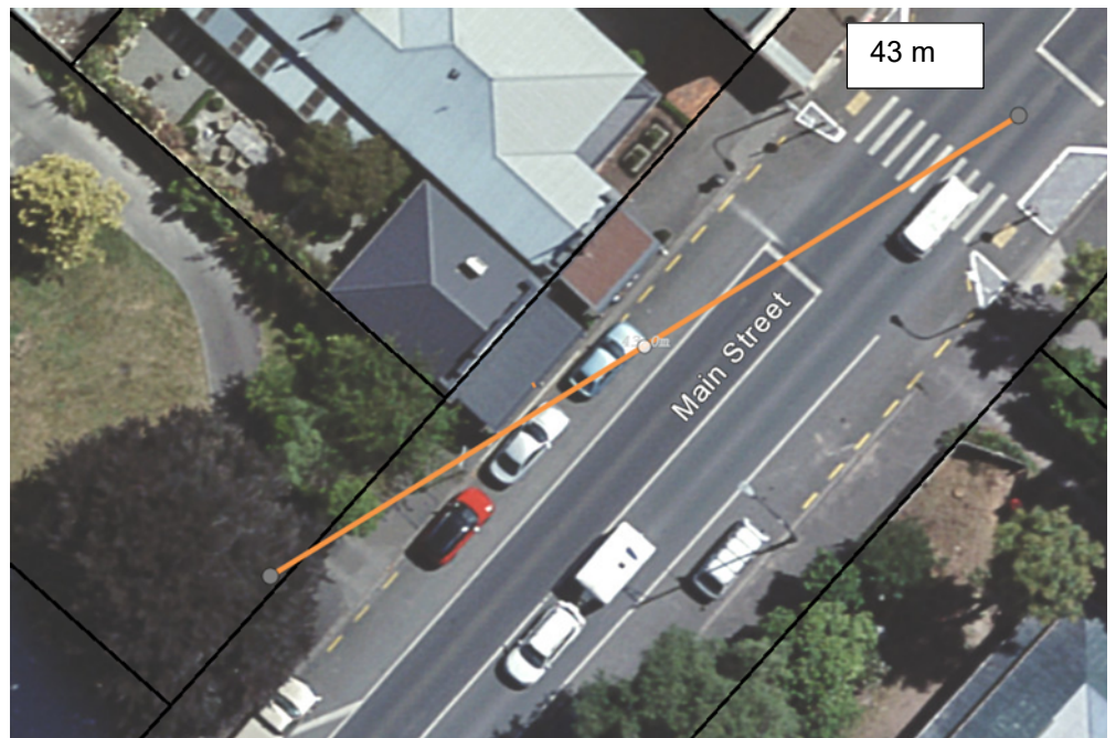
Figure 3: No Right Turn visibility inadequate
