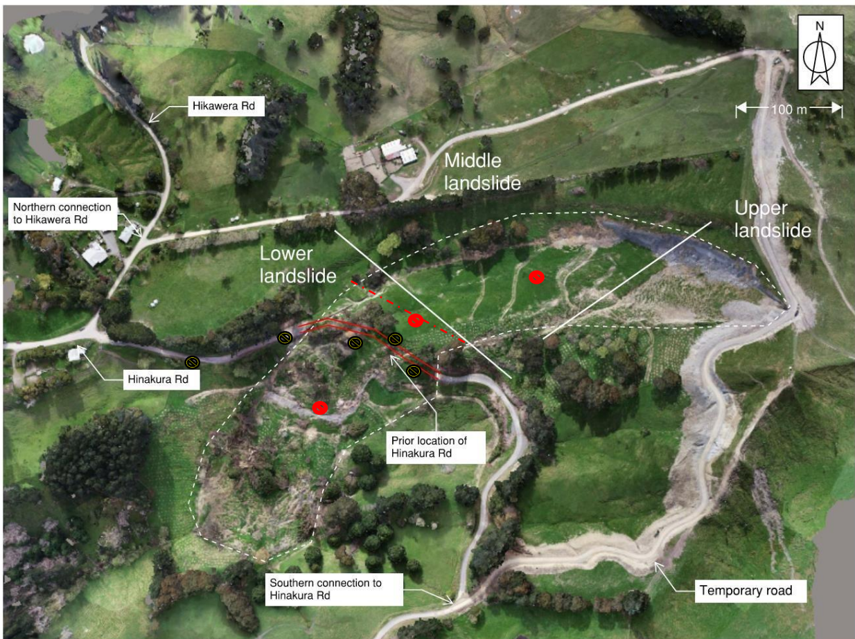
Figure 3: Provisional borehole locations (8) and Geophysical line. Red investigations are deep to investigate landslide depth. October 2022 base photo showing translated road pavement.
